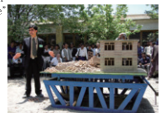
Shake table demonstration of building models (retrofitted and non-retrofitted) in Afghanistan
