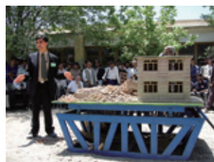
Shake table demonstration of building models (retrofitted and non-retrofitted) in Afghanistan
